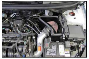
13. Connect the factory vent lines to the hoses connected to the K&N<sup>®</sup> intake tube.
