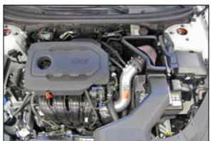
14. Reinstall the decorative engine cover. Install the factory fresh air intake duct into the K&N<sup>®</sup> heat shield and core support.
