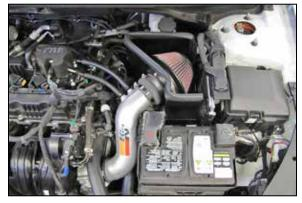
12. Using the provided coupler hose (084079) Install the K&N<sup>®</sup> intake tube into the vehicle, adjust the tube for best fit and then secure with the provided hose clamps.
