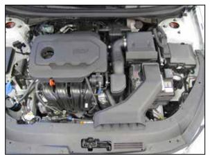
2. Lift off the decorative engine cover. Remove the fresh air intake duct from the factory air filter housing and core support.
