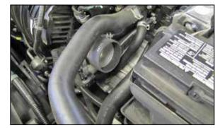
6. Install the provided coupler (08711) into the throttle body and secure with the provided hose clamp.
