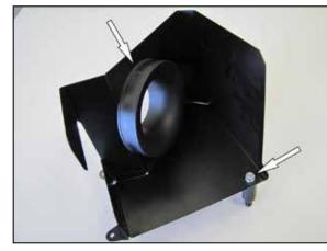
8. Install the filter adapter into the heat shield and secure with the provided hardware. Install the heat shield mount onto the heat shield using the provided hardware.
